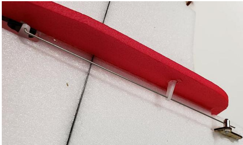
Servo arm, rod, standoff, linkage stopper and plywood horn installed
