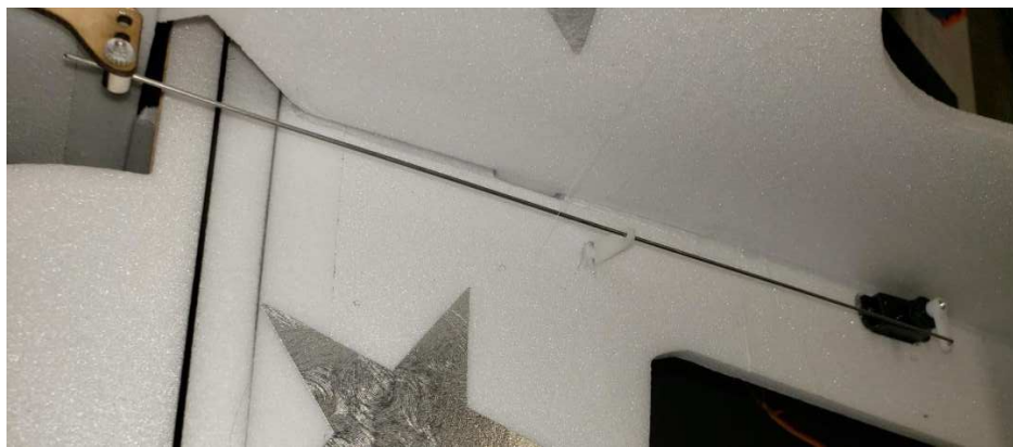
Rudder horn/linkage stopper/standoff installation
