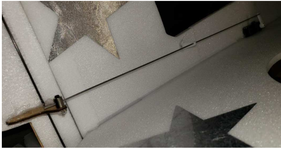
Elevator horn/linkage stopper/standoff installation
