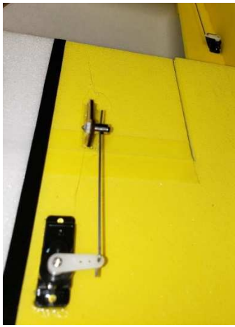
Aileron horns/linkage stopper installation
