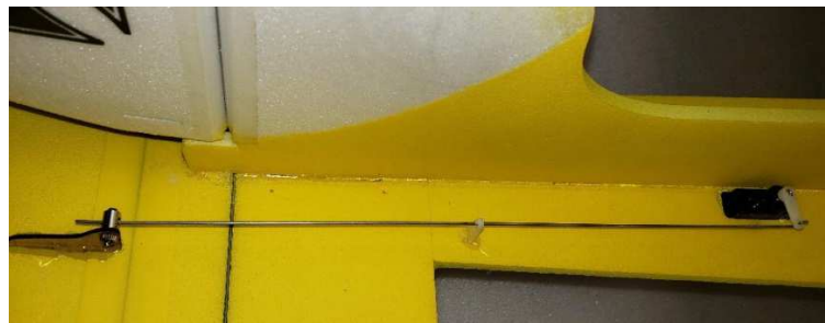
Elevator horn/linkage stopper/standoff installation
