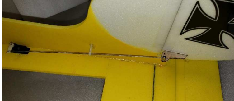
Rudder horn/linkage stopper/standoff installation
